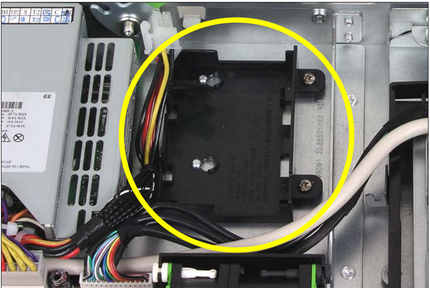
Figure 31: Position of the iBBU holder in the server
